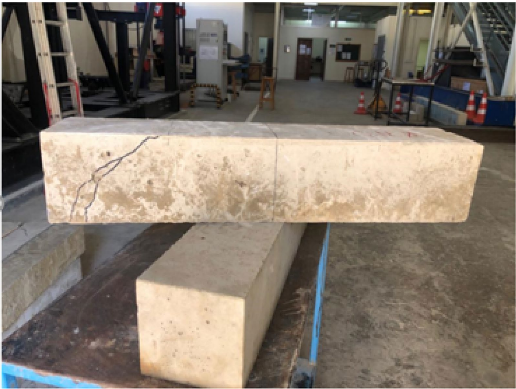
Fig. 11 RC beam shear reinforced with stirrups
