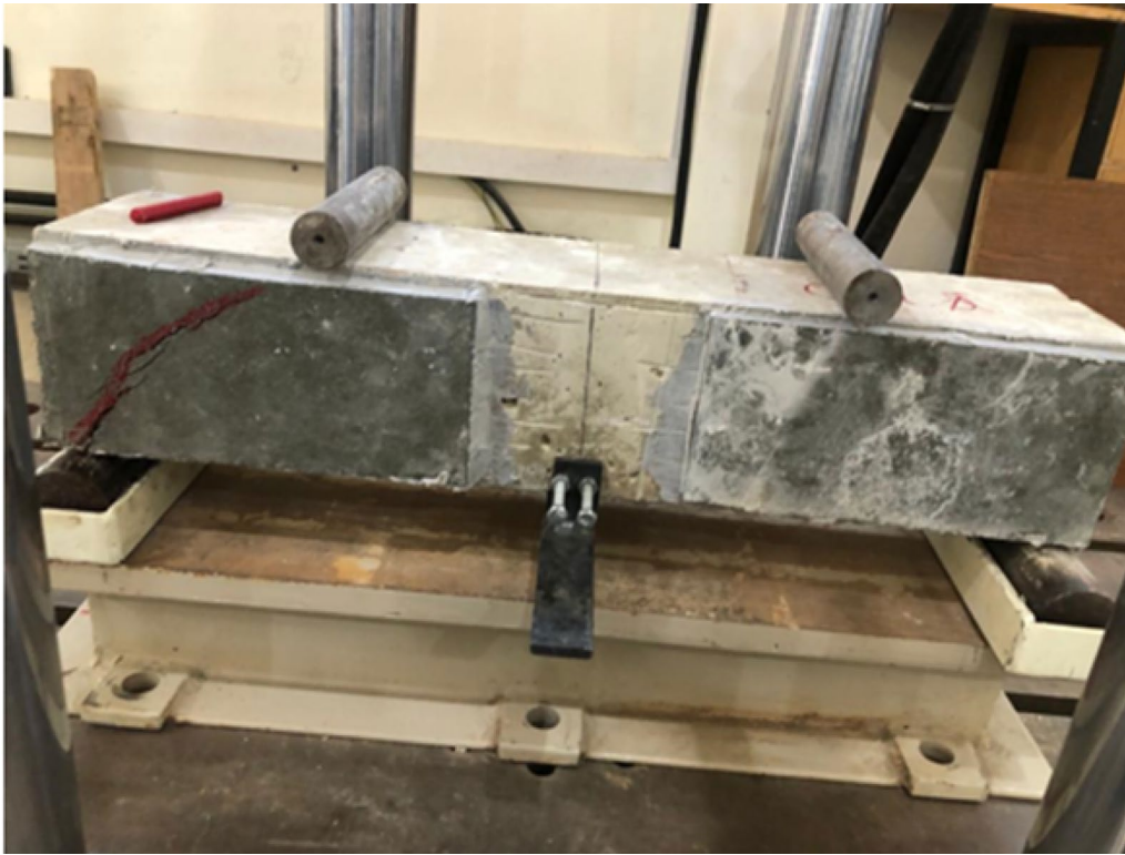
Fig. 13 RC beam without stirrups strengthened with HPFRC plates
