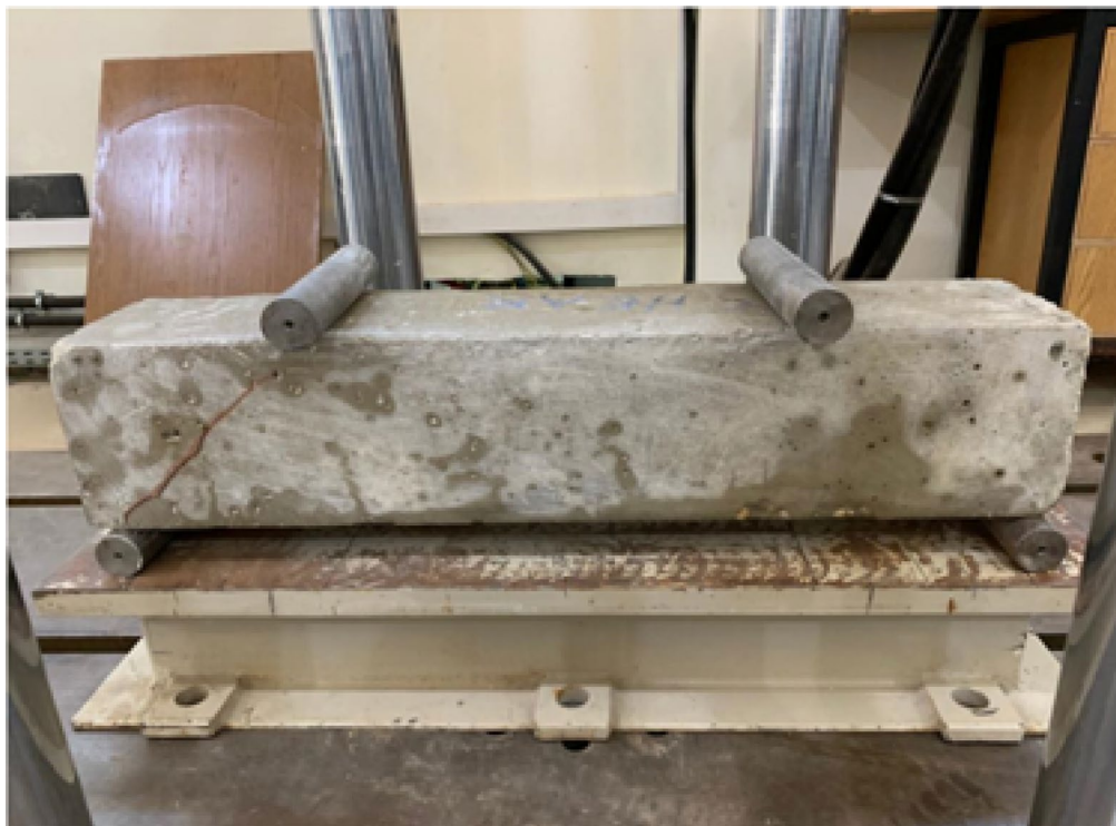
Fig. 10 Reference RC beam without stirrups
