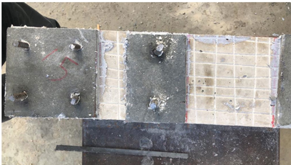
Fig. 8 Strengthening scheme with HPFRC strips
