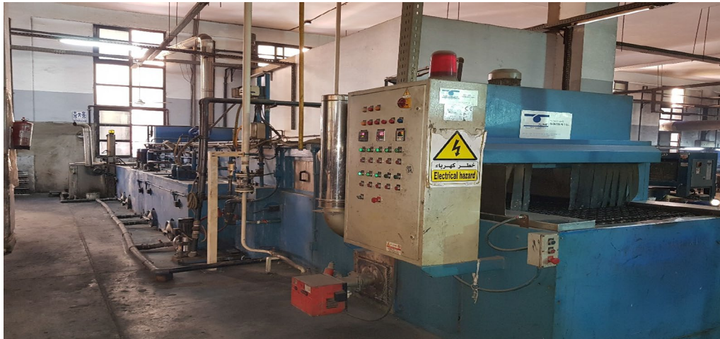
Fig. 1 Pots washing machine using NaOH solution in Nouval factory, Badr city
