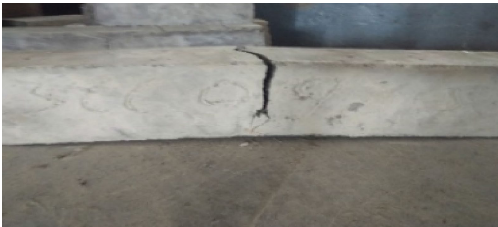
Fig. 11 Bridging effect of fiber (Sanjeev & Nitesh, 2020)
