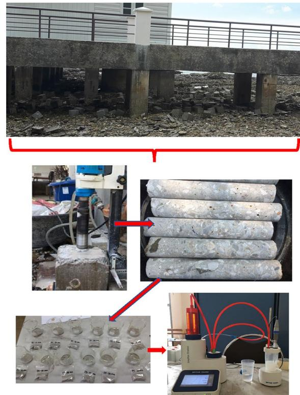
**Fig. 1** Specimen preparations and chloride content measurements in the concrete
