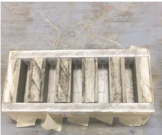
Fig. 3—Forty mm (1.57 in.) mold with fibers installed.
