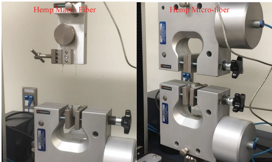
Fig. 4—Tension testing configuration.
