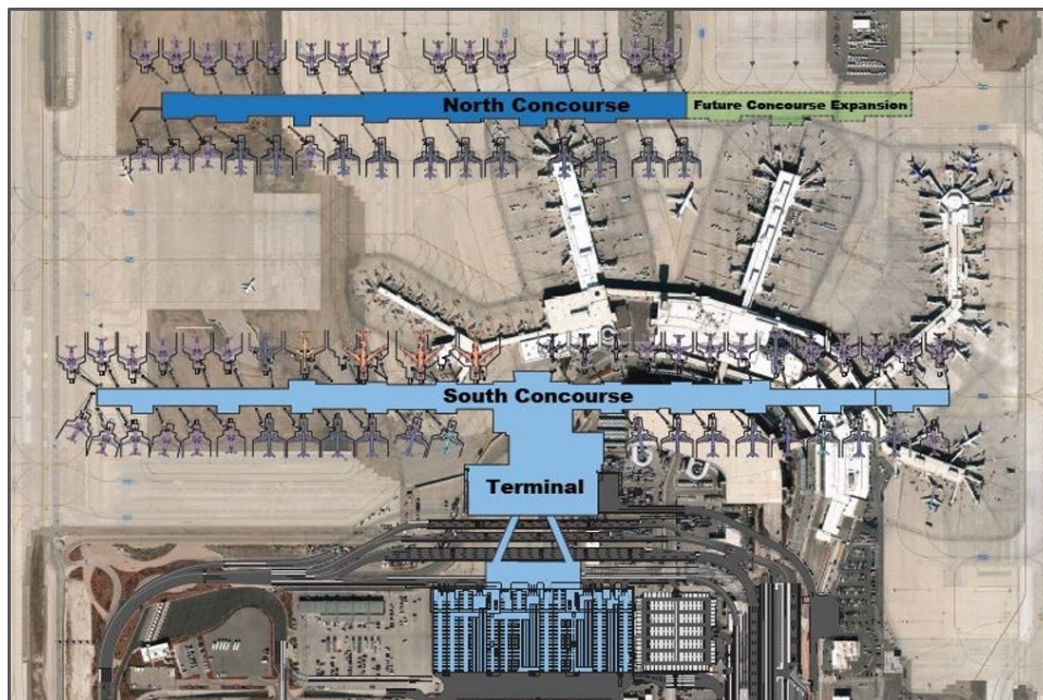
Figure 1-3 Location of new SLC airport terminal, concourses, and parking garage (all in blue) superimposed over the location of the old SLC airport and parking garage (in white or tan). The new airport's south concourse will be through the location of the parking garage, hence why it will be demolished.
