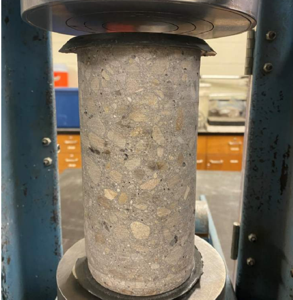
Figure 3-21: Compressive strength testing.
