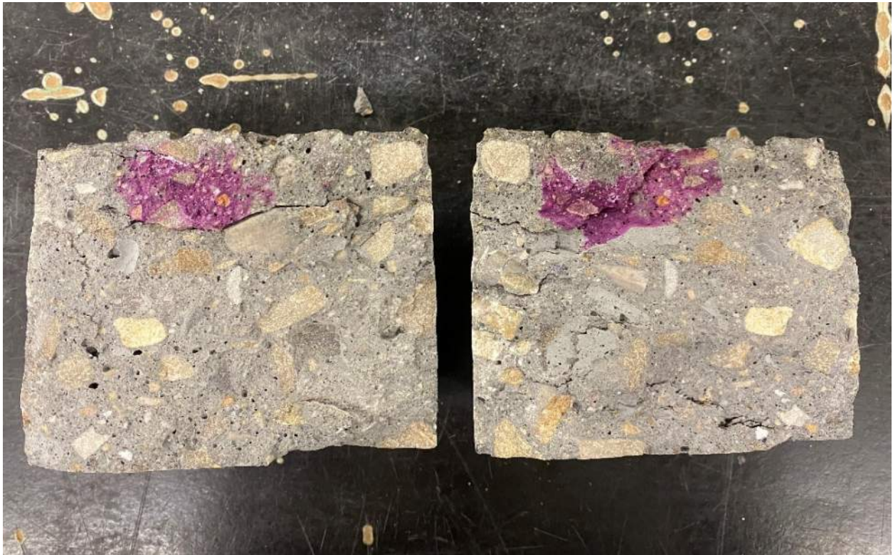
Figure 3-22: Carbonation depth testing.
