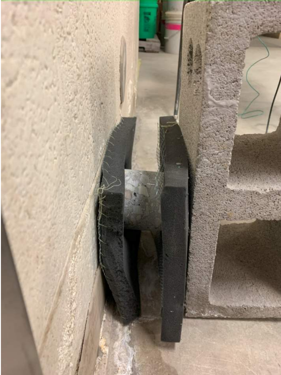
Figure 3-18: Electrical impedance testing.
