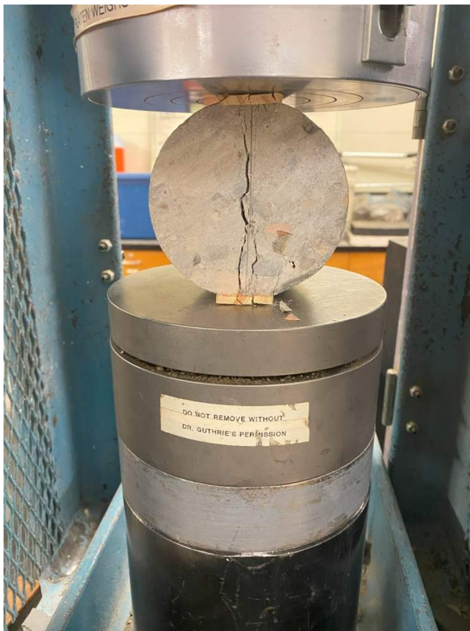
Figure 4-1: Typical core after splitting tensile strength testing.
