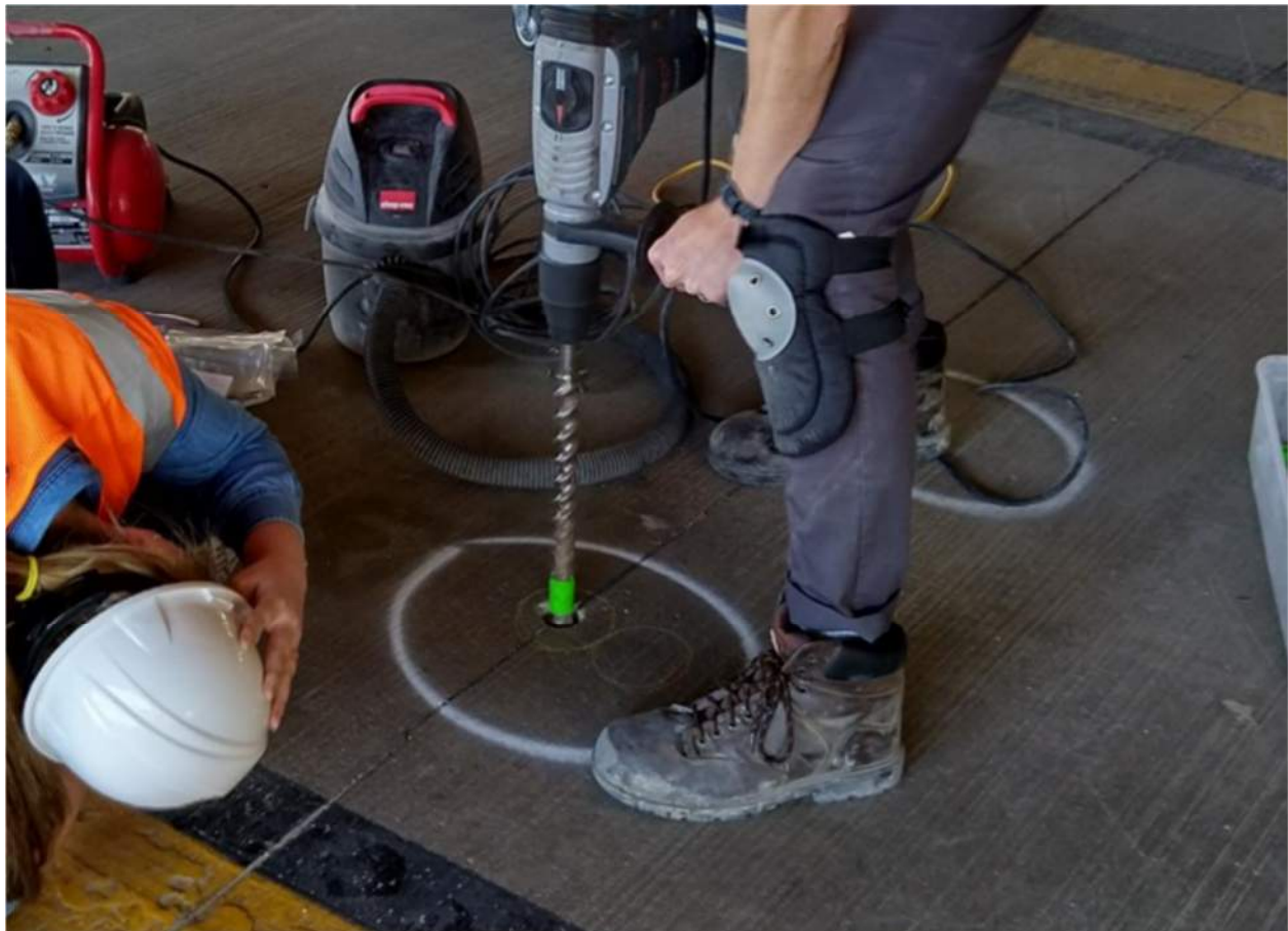
Figure 3-14: Chloride concentration sampling.
