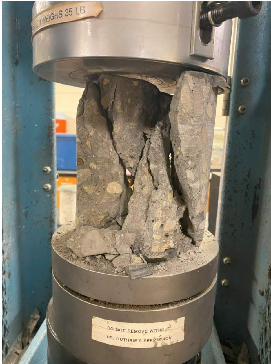
Figure 4-2: Typical core after compressive strength testing.
