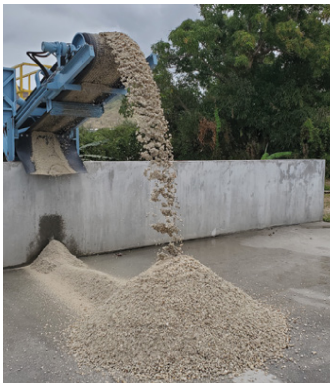
Reclaimed sand and aggregate from the JADAIR Redi-Wash Washout System
