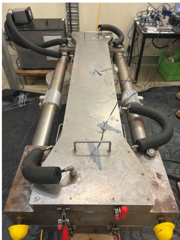
Fig. 3 Test of rigid cracking frame
