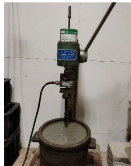
Fig. 3 Determination of the vertical expansion rate
