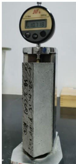
Fig. 10 Determination of restricted and free expansion rate
