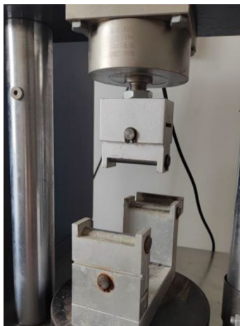
Fig. 5 Flexural strength test
