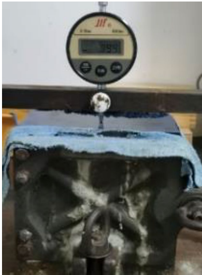
Fig. 4 Determination of setting time
