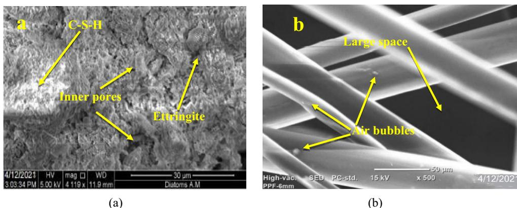
**Fig. 13** SEM image of **a** optimum strength specimen, **b** lowest strength blended specimen
