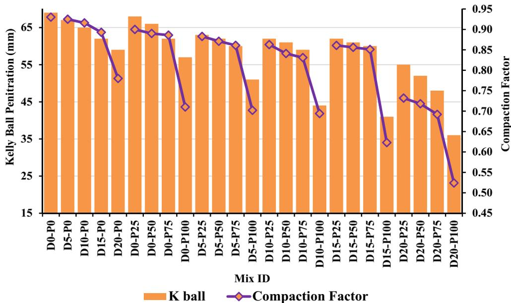
**Fig. 4** Kelly ball penetration and compaction factor
