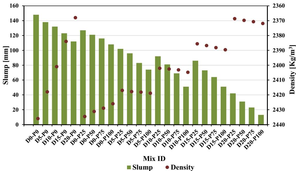
**Fig. 2** Slump and density of different concrete mixers
