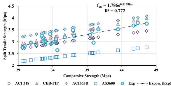
**Fig. 8** Analytical relationship between compressive and split tensile strength
