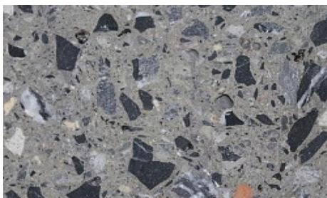
**Fig. 10** Diamond-blade-cut sample of  $D_{15}-P_{75}$  after water penetration
