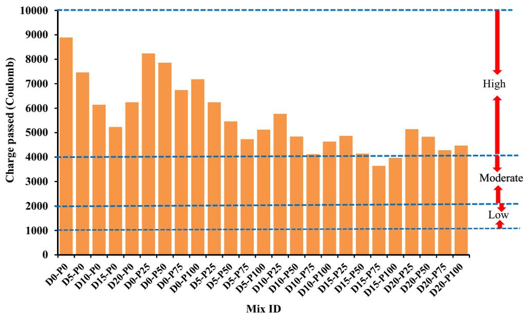
**Fig. 11** Rapid chloride penetration test result
