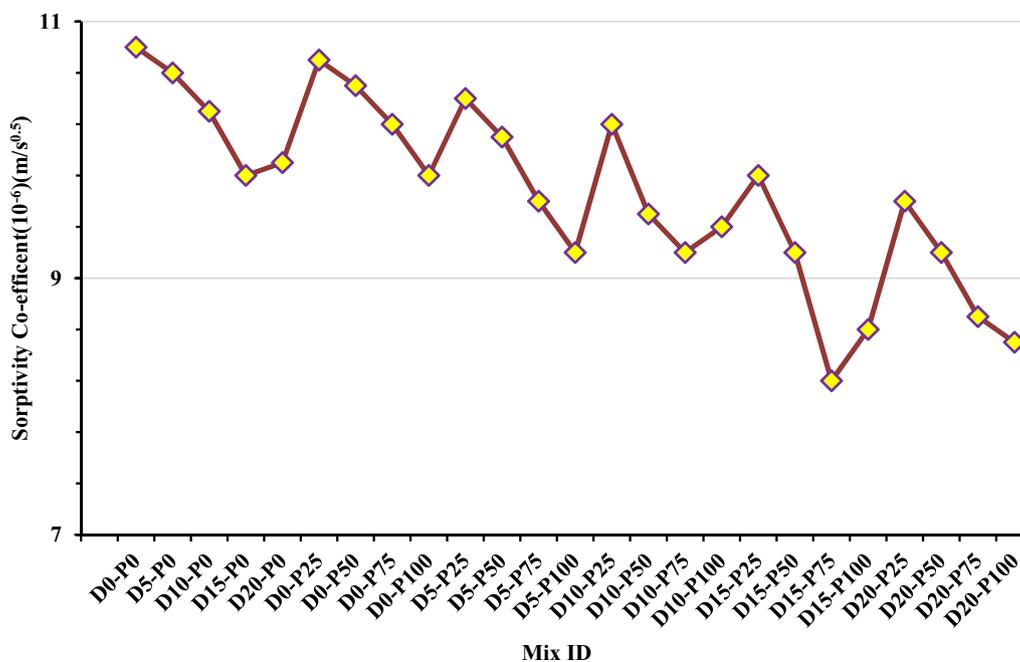
Fig. 12 Sorptivity co-efficient test result
