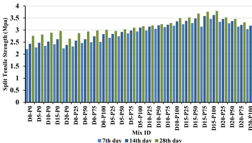
Fig. 7 Split tensile strength of different replacements
