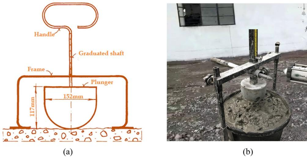
**Fig. 3** a Kelly ball apparatus schematic, b Kelly ball test on DE with PPF sample
