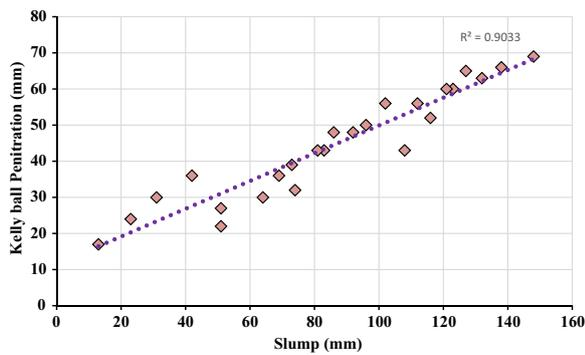
Fig. 5 Relation between ball penetration and slump value
