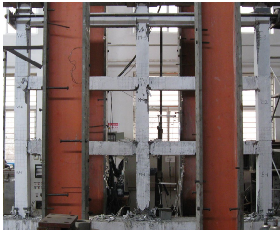
Fig. 4 Failure mode of SRUHSC frame specimen
