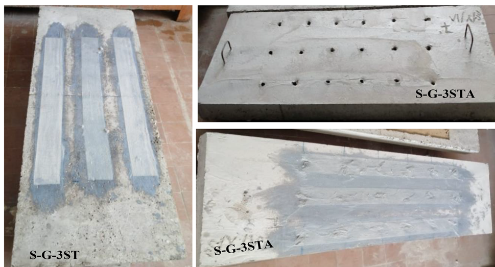
(a) Slabs strengthened by EB- technique (without/with) anchors
