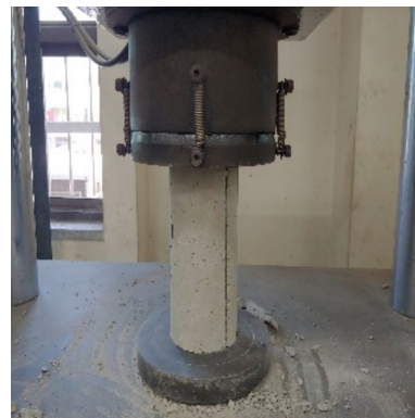
Fig. 3 Concrete compressive strength test
