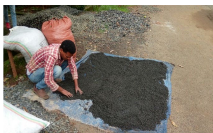
a. Fine steel slag after screening and washing
