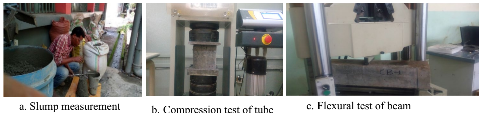
Fig. 3 Slump measurement, compression test of cube, and flexural test of beam
