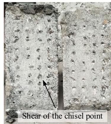
**Fig. 7** Shear failure of UHPC bulge at the chisel point
