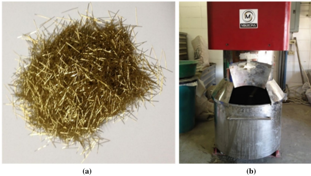
Fig. 2 a Micro copper coated steel fibres; and b Planetary mixer
