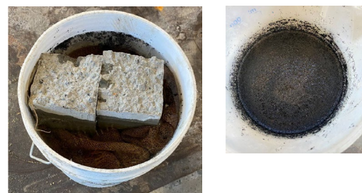
Fig. 2 Soaking rubber in water for 24 h
