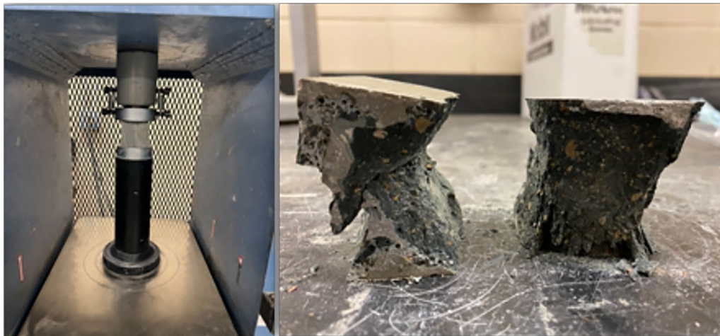
Fig. 4 Test setup for 2-inch cube compressive strength
