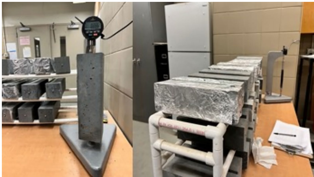
Fig. 6 Drying and autogenous shrinkage samples (covered with aluminum foil to prevent moisture loss)
