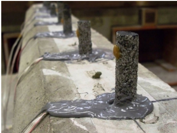
Fig. 3 Embedded through-section FRP bar shear-strengthening technique
