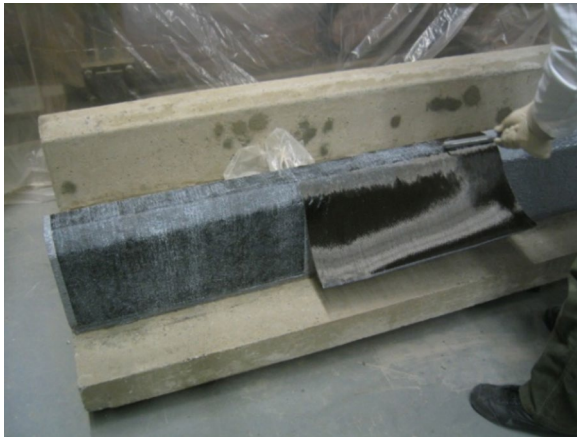
Fig. 1 Externally bonded (EB) FRP sheet shear-strengthening technique
