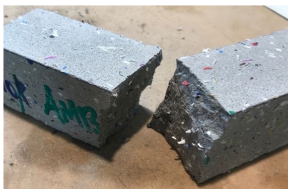
Fig. 12. 3D-printed flexural sample plastic alignment
