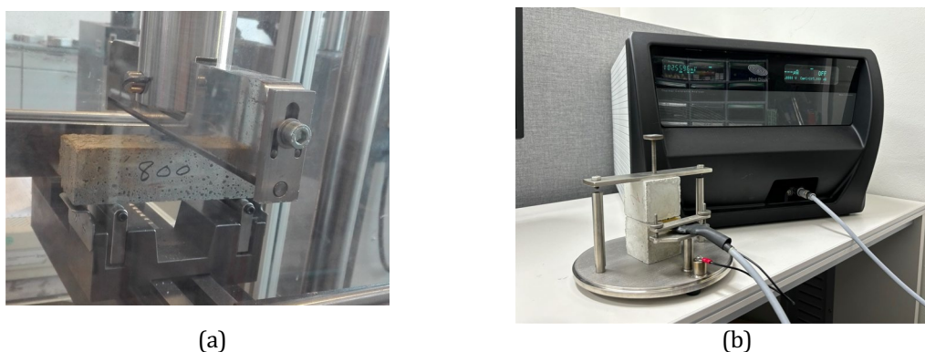
Fig. 3 Measurement of material properties: a flexural strength measurement, b thermal property evaluation using a hot disk
